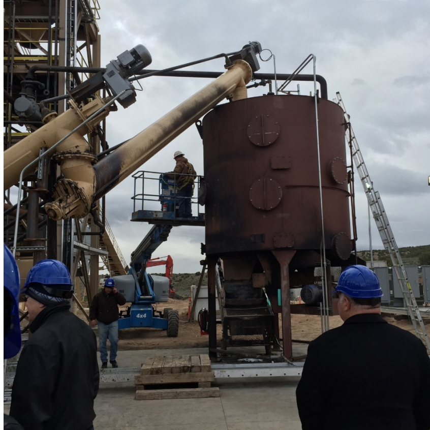
Figure 3. MCW oil sands drying vessel in Maeser, Utah. The post processed sands are heated with steam to vaporize any remaining solvent in the sand. All vaporized solvent is collected, condensed and returned to the closed loop system to start the process over again. This process recovers over 99% of the solvent for reuse.
