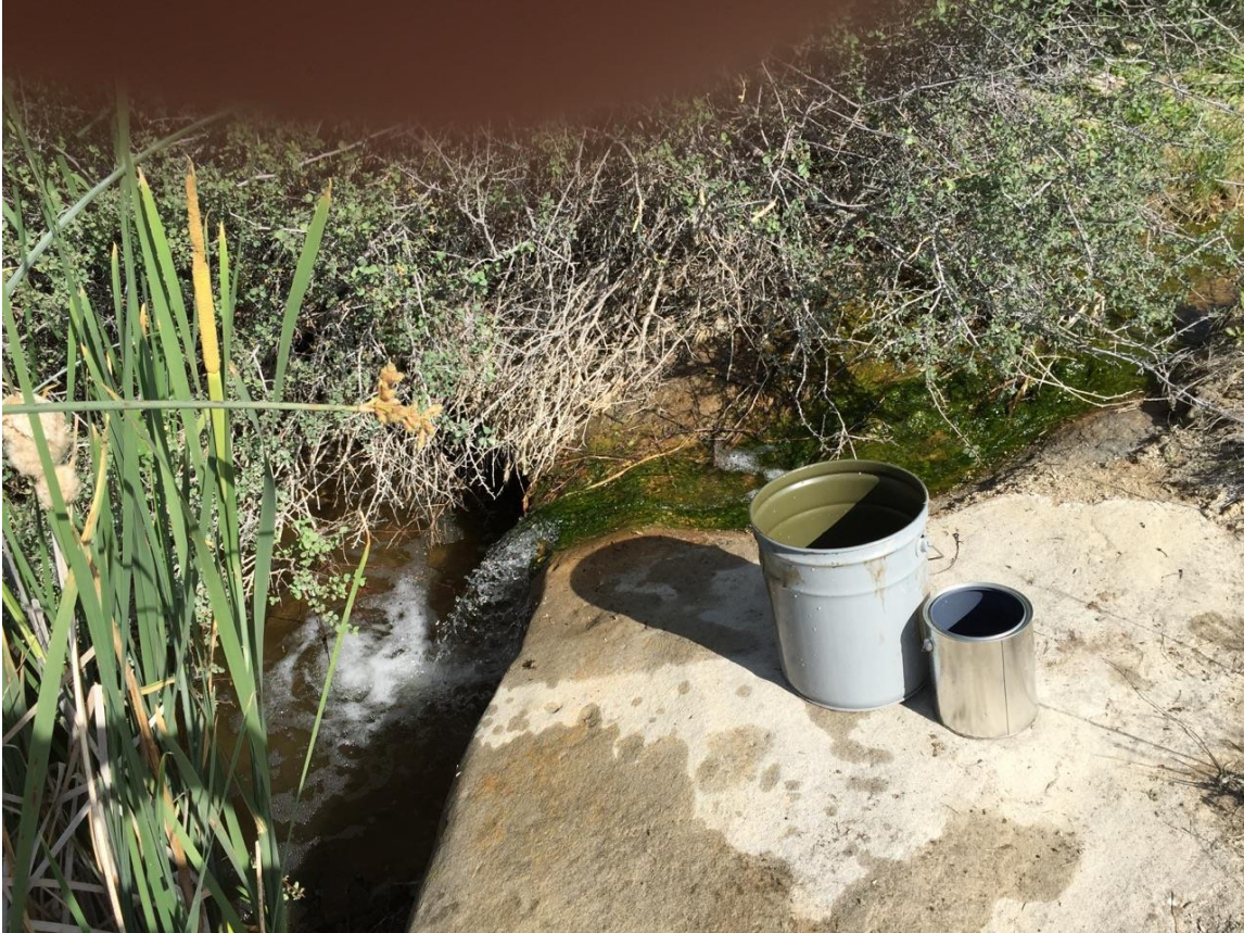
Photograph P15. Intermittent stream 1 (identified by the URS Corporation (2008) in figure 4) near the eastern border of the survey area. Stream flow was measured using the bucket method at this location. Elevation 5020 feet. See figure 3 for location of picture.
