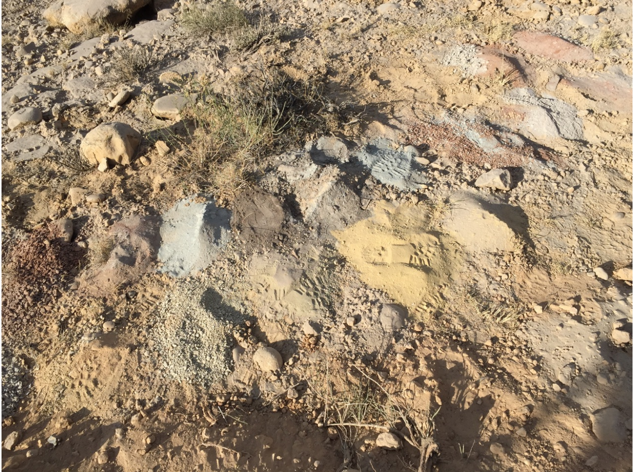
Figure 5. Cutting from the ground water monitoring well that was drilled approximately 100 feet to the east of well CF-1. Air rotary drilling produced cuttings that were exceptionally dry and easy to identify. The majority of cuttings were from interbedded red and gray shales. The black cuttings near the center of the picture are oil sands. No water was encountered at the two target zones at 58.1 - 60.7 feet and 215+ feet.
